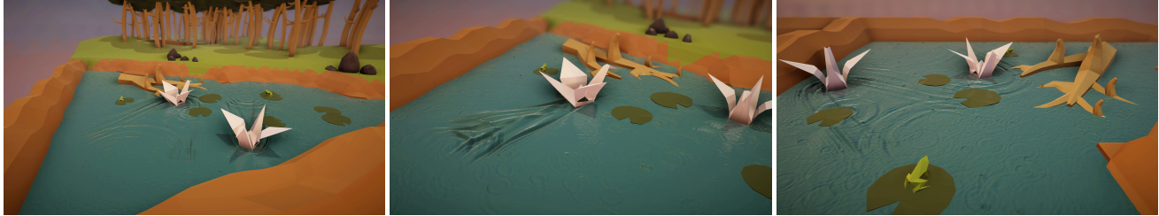
Figure 1: Rain on the pond. Our wave simulation method captures the gravity waves present in the wakes produced by the paper birds, as well as the capillary waves produced by rain drops, all with correct scale-dependent velocities. The waves reflect on all the objects in the scene, both static and dynamic. The domain is 4 meters wide, and is simulated on a 1024 \times 1024 grid, at just 1.6 sec. per frame.
