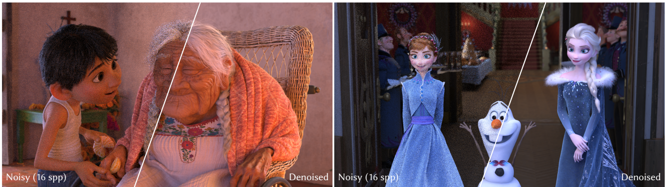
Fig. 1. We introduce a novel, modular architecture based on kernel-predicting neural networks that performs multi-scale, temporal denoising of rendered sequences. Our network can be retrained using a small amount of data and performs robustly with artist-control over the variance-bias tradeoff on novel data, such as these two examples from our test set. © Disney / Pixar, © Disney.
