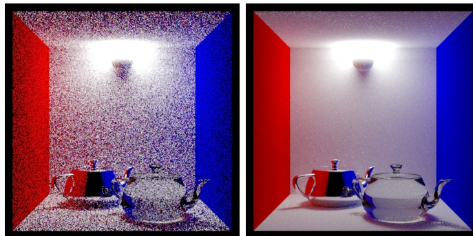
Figure 8.2: Unidirectional vs. bidirectional path tracing in a scene dominated by indirect illumination. Equal time renderers (2048 vs. 600 samples per pixel).
