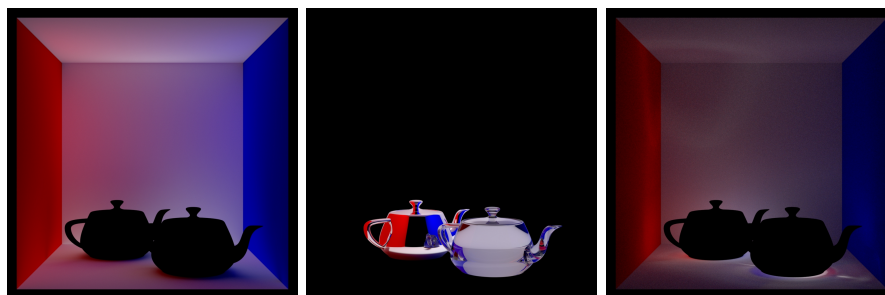
Figure 2.2: Indirect illumination components: (a) Indirect diffuse. (b) Specular reflections and refractions of diffusely reflected light. (c) Diffuse reflection of specular reflections and refractions (caustics).
