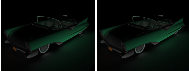
Figure 6: Color bleeding on a NURBS car and ground plane. (a) Ray-traced image. (b) Point-based image.
