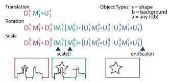
Figure 2. Regular expressions for translation, rotation and scale gestures. The thumbnails illustrate the user's actions corresponding to the colored symbols for the scale gesture.
