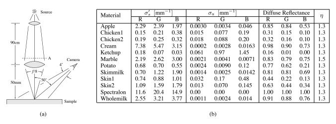
Figure 5: (a) Measurement apparatus, (b) measured parameters for several materials.
