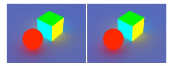
Figure 3.9: Color bleeding computed using gather. (a) 16 samples; (b) 256 samples.
