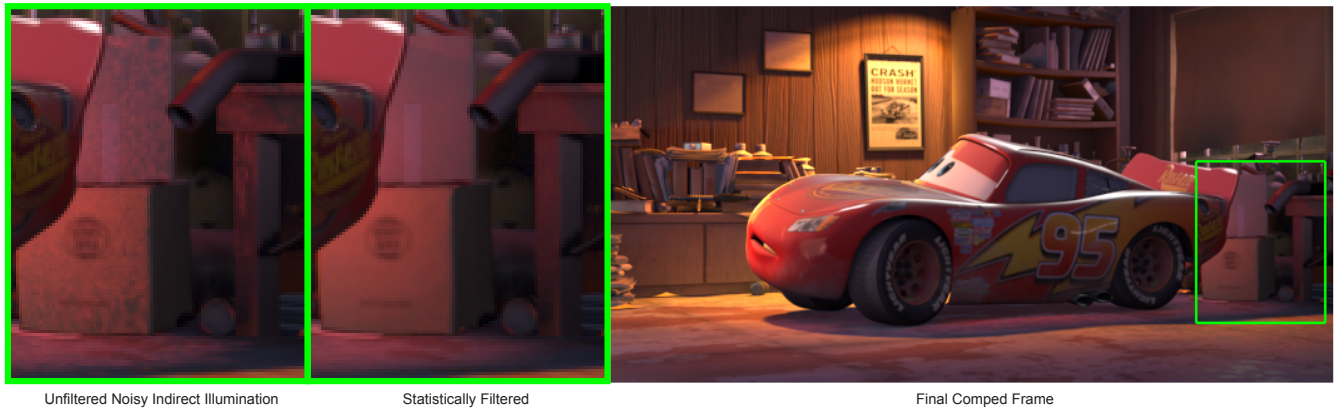
Figure 1: An example of our statistical acceleration technique on a production shot: Our technique accelerates rendering by quickly computing noisy, low sample indirect illumination and using the variation over time to statistically denoise it. The left image shows a zoomed view of the shot using the noisy, unfiltered indirect illumination while the middle image uses the statistically filtered indirect illumination (contrast has been enhanced slightly to better illustrate the noise in print). The rightmost image shows the final comped frame using the statistically filtered indirect illumination. See the video for the full animation sequence.
