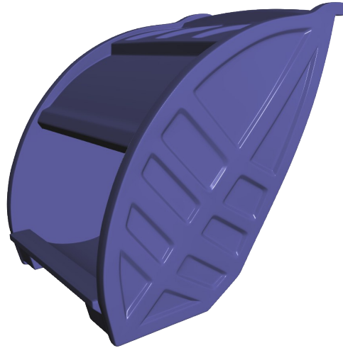
Figure 11: A shape modeled with semi-sharp creases
