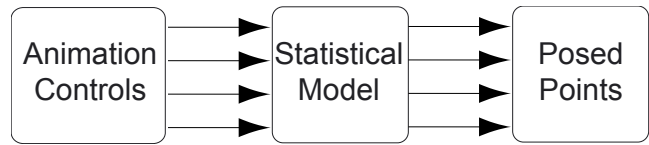
Figure 2: Block Diagram of a basic statistical modeling system for animation: The trained statistical model accepts as input the animation variables and produces the posed points as output. Unfortunately, since the relationships between the animation variables and the posed points can be extremely nonlinear, both the statistical model as well as the training set must account for these complex nonlinearities.
