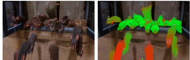
Figure 14: In the left image, simplification depends on motion blur. In the right image, color indicates \lambda_{blur} : green areas are more detailed, red areas are more simplified.
