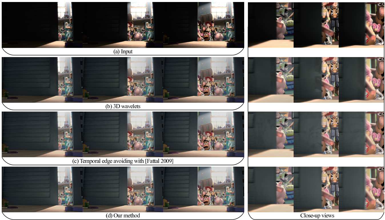
Figure 6: Ghosting artifacts. (a) Three of the input HDR frames displayed in linear color space. (b) Tone mapped frames using 3D wavelet based algorithm (without temporal edge avoidance). (c) Tone mapped frames of applying edge avoiding wavelets from [Fattal 2009] in time. (d) Our results with temporal edge avoiding wavelets. Close-up views are shown on the right. Ghosting artifacts can be observed through the sliding door in (b) and (c).
