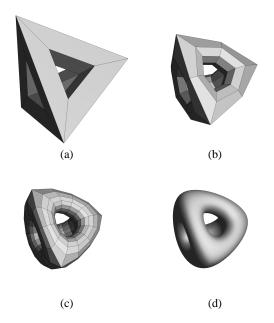
Figure 3: Recursive subdivision of a topologically complicated mesh: (a) the control mesh; (b) after one subdivision step; (c) after two subdivision steps; (d) the limit surface.
