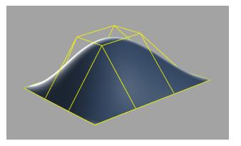
Figure 6: A surface where boundary edges are tagged as sharp and boundary vertices of valence two are tagged as corners. The control mesh is yellow and the limit surface is cyan.
