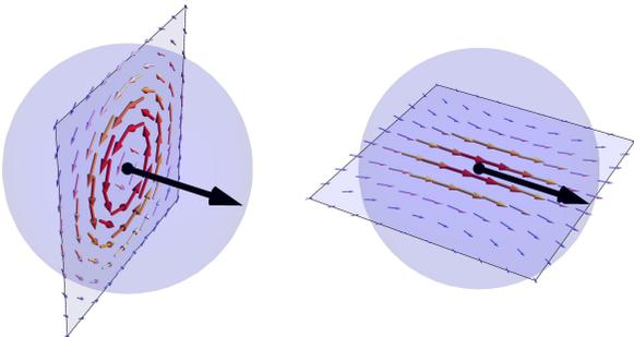
**Figure 2:** Left: slice of the velocity field induced by a vorticity. Right: slice of the vorticity field induced by a vorticity.
