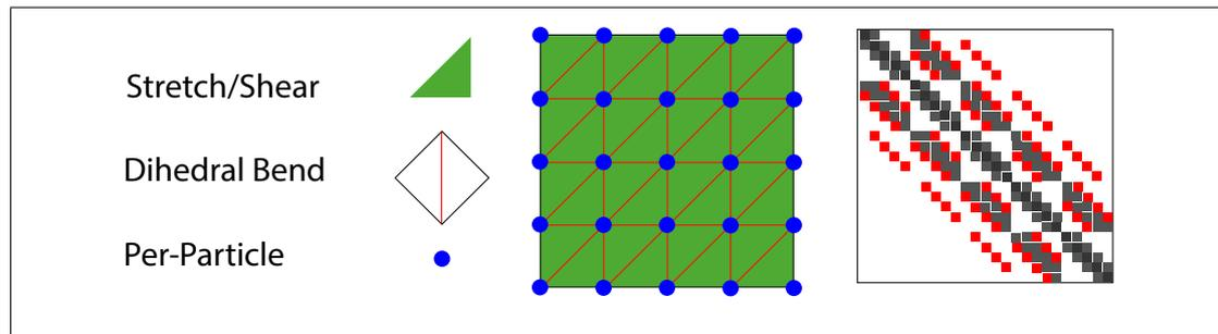
It makes sense to at least group the element forces by their mesh component domains, but we can go further. Instead of having a force element that handles each type of mesh feature, we aggregate overlapping forces onto the same fixed force element. Some elements naturally will be responsible for more force types than others and some will remain isolated.
