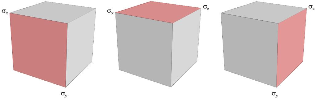
Figure 5.3.:  $II_C^*$  sums up the squared *areas* of each side of the cube:  $II_C^* = (\sigma_x\sigma_y)^2 + (\sigma_x\sigma_z)^2 + (\sigma_y\sigma_z)^2$ . I.e. it measures the overall face areas of the entire cube.
