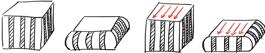
Figure 8.2.: **Left pair:** An isotropic material bulges out equally in all directions **Right pair:** Fiber reinforcement has been inserted, so it bulges less in that direction. The lines along the front remain vertical.
