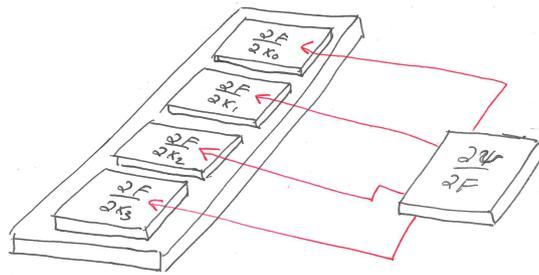
Figure 3.3.: Double-contraction of a 3<sup>rd</sup>-order tensor against a 2<sup>nd</sup>-order tensor is like taking a cheese slice (right) and double-contracting it against each slice on the cutting board (left). The result here would be an  $\mathbb{R}^4$  vector.
