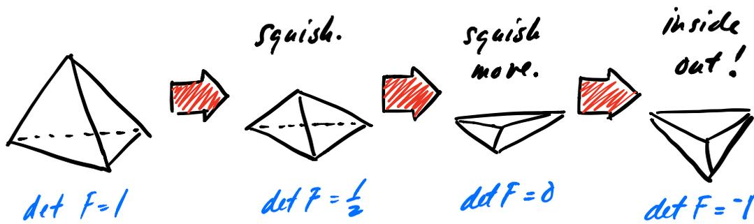
Figure 6.1.: A tetrahedron is sitting on a table (left). We squish its top vertex down (center, left) until it has been smashed into a pancake (center, right). We keep pushing, and the tetrahedron flips inside out! This is not physically possible, but it can happen numerically.
