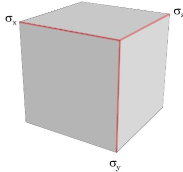
Figure 5.1.: The matrix  $\mathbf{F}$  describes the rotation and scaling of an infinitesimal cube of material. The singular values of  $\mathbf{F}$ , the  $\sigma_{\{x,y,z\}}$  labels above, describe the lengths of each side of that cube.
