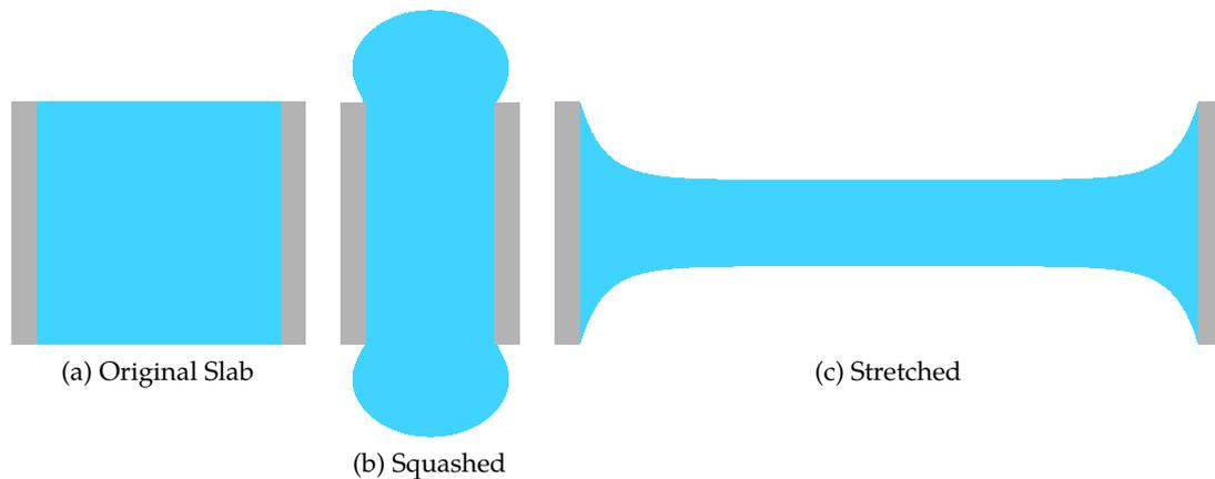
Figure 6.3.: What we want from a 2D square of rubber (left). Under squashing, stuff squeezes out the top and bottom (center). Under stretching, it swoops down to a nice clean line along the middle (right).
