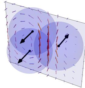
**Figure 3:** A velocity field is induced by multiple vortices, illustrated with three vortices orthogonal to a plane.
