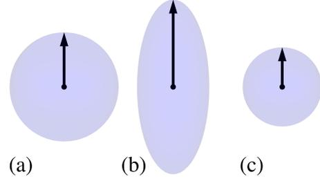
**Figure 4:** A vorticle (a) is stretched into vorticle (b): the mean energy is preserved while the enstrophy changes. Vorticle (b) is then resampled in an unstretched vorticle (c) with the same mean energy and enstrophy as vorticle (b).
