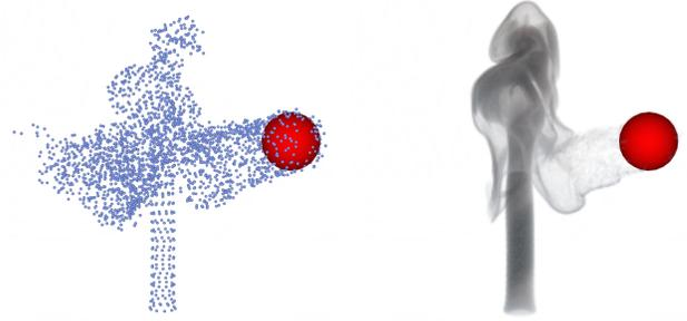
**Figure 8:** Left: 2400 vorticles, showing the vertical current and the collider's trail. Right: advected densities. Dynamics can be limited to the visible areas simply by deleting points.
