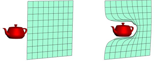
**Figure 6:** Left: initial position of a boundary object (red) moving into points (green lattice). Right: the harmonic field warps space in an incompressible and irrotational manner, with a slip boundary.
