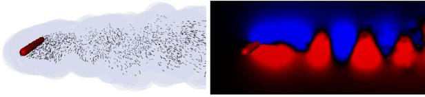
**Figure 7:** Left: a constant flow moves at  $10\text{m}\cdot\text{s}^{-1}$  with  $\nu = 0.1$  around a static pole of radius 1 (red): the surface sheds vortices (black arrows). Right: a slice of the vorticity induced by the vortices reveals the emergent behavior of a von Kármán vortex street.
